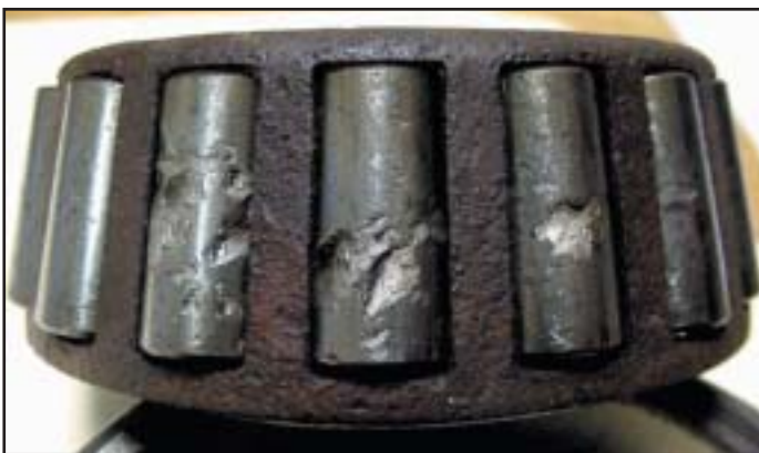
Spalling, or breakdown, of a bearing's tapered rollers can be caused by excessive loading or improper lubrication.
