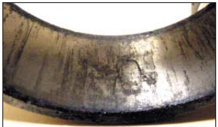
Pitting or erosion of the mating bearing cup can result from excessive loading or improper lubrication.
