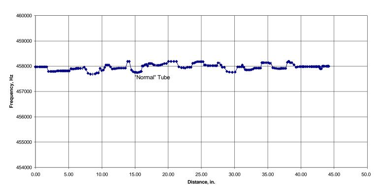
The third plot is of a .625" diameter copper tube with surface nicks the nicks are evidenced by the drops in the resonant frequency. Although this data was recorded with a rather low resolution RM-EMAT the areas of where heavier defect clusters are located significantly affect the resonant frequency for this tube. A higher wavelength count transducer will provide less dispersion of the acoustic waves and thus will yield greater spatial resolution and finer detail.
