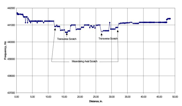
This first chart details the resonant frequency of a .5 "diameter copper tube with a .025" nominal wall thickness. This sample had several transverse scratches with a long meandering axially oriented scratch. The ends of the tube were relatively free of visible defects.
