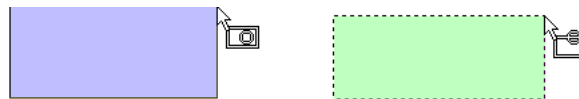
BricsCAD uses colors and icons to report the style of a windowed selection:
