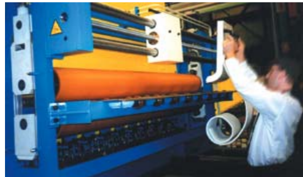
Figure 2 With this hands-off roll cleaning device, a small coil of cleaning media is placed between the slowly turning work rolls. The machine then moves it back and forth across the face of the rolls.
